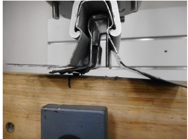
FIG.3 CONCEALED CLIP SCREW DEFORMATION
