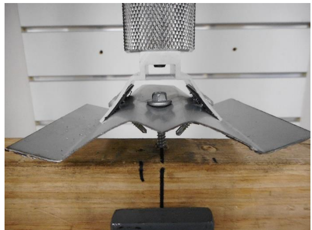
FIG.5 TRIMDEK ROOF SHEET DEFORMATION
