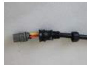
▲ Figure 4.16 Connect Wires to the Terminal
